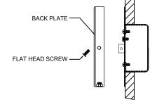
**5.** Attach the fixture to the mounting ring w/ wing and secure it with flathead screws. (See Figure-02)
